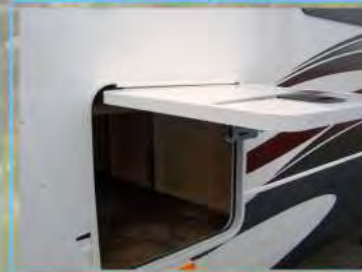
1" Thick Thermal Insulated Luggage Door Compartments
