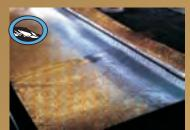
We use Astro-foil (R-15) insulation along the entire length of the floor. Plus an additional wrap around the holding tanks
