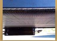
In a 4 Seasons Outdoors enclosed from front to pack for both insulation and protection from road debris.
