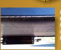
In a 4 Seasons TimberRidge the entire chassis is enclosed from front to back for both insulation and protection from road debris.
