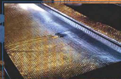
R-15 Astro-Foil Roof, Slide-Out Floor, Entire Underbelly, Additional Wrap Around Holding Tanks
